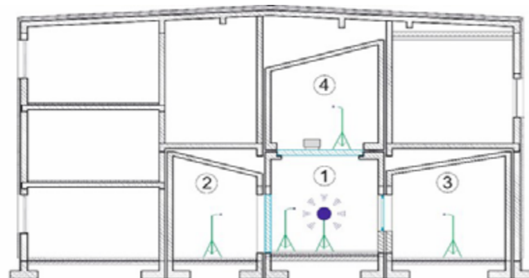
1 – transmitting-receiving chamber, 2, 3 – receiving chambers, 4 – transmitting chamber
